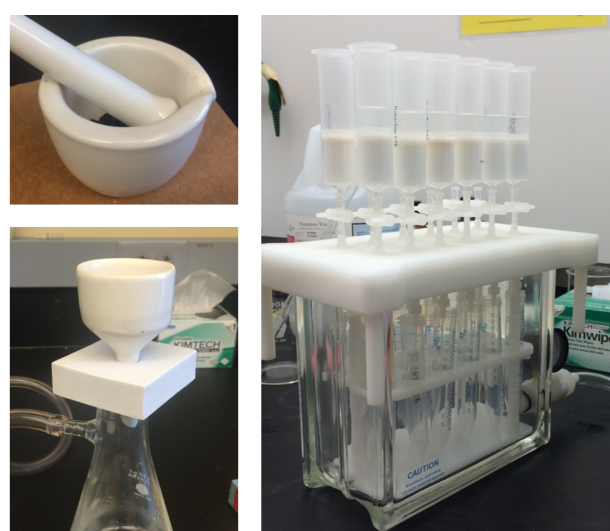
Figure 2. Procedure involves grinding seeds and multiple washes with ethanol, methanol, and hexane.
